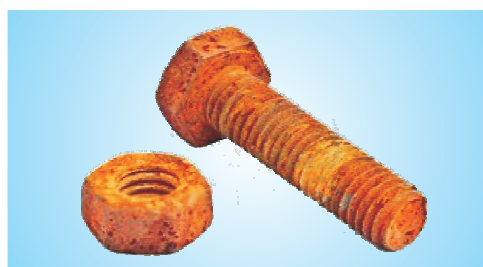
Fig. 4.9: Rusted nuts and bolts of iron
