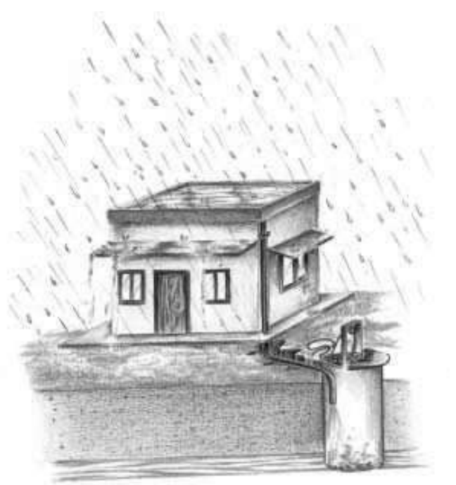
(b) Recharge through Abandoned Dugwell
