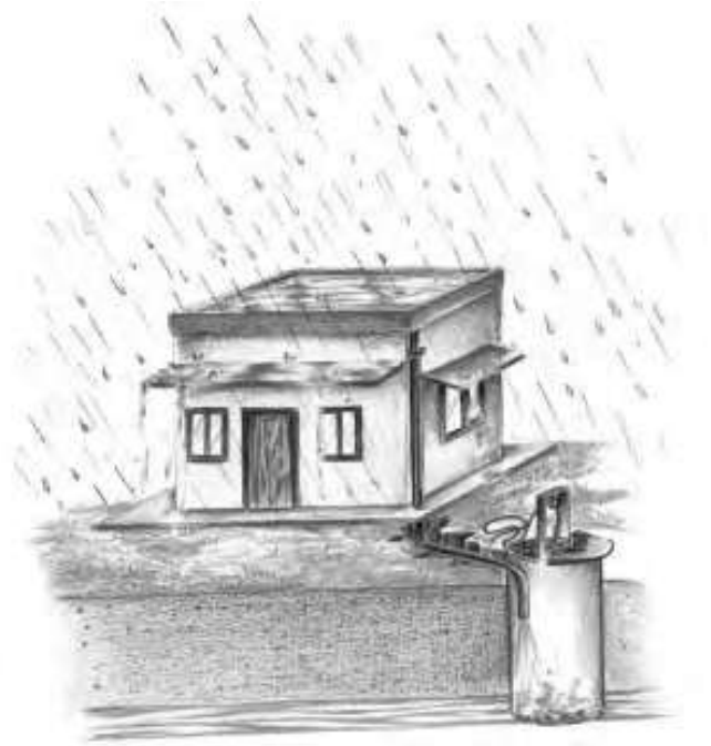
(b) Recharge through Abandoned Dugwell
