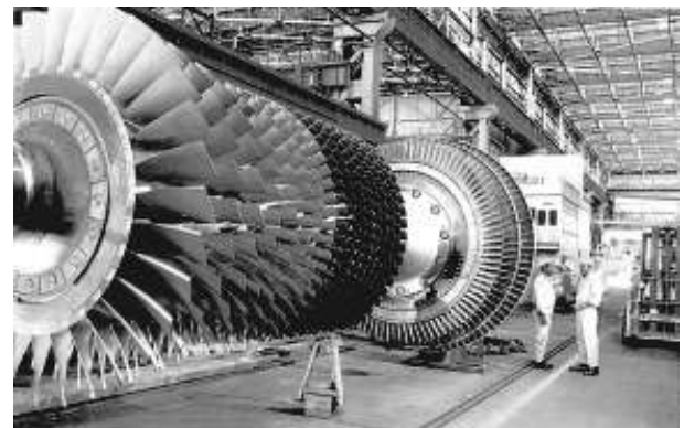
Fig. 6.10: Gas turbine rotor on assembly bed at BHEL, Hyderabad
