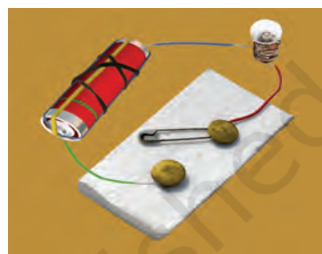
Fig 12.9 An electric circuit with a switch
