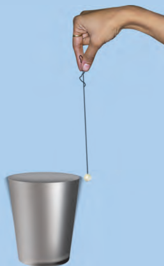
Fig. 13.17 : Thermocol ball touching the vibrating glass tumbler
