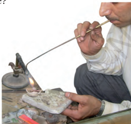
Fig. 6.14 : Goldsmith blowing through a metallic pipe
