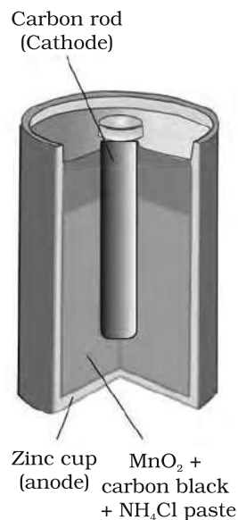
Fig. 3.8: A commercial dry cell consists of a graphite (carbon) cathode in a zinc container; the latter acts as the anode.
